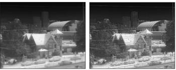
SHARPNESS -20 SHARPNESS +100 FIGURE 3-18. SHARPNESS CORRECTION
