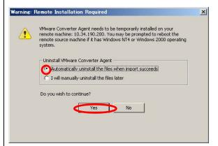
21 The VMware Converter Agent will start being installed on your source machine.
