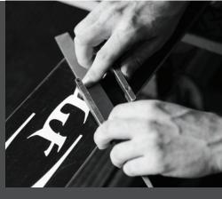
work properly. Tip: run a sharpie the entire length of the edge prior to filing. By doing so, one can see how much material is being removed.
