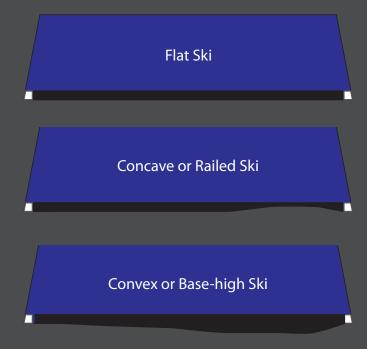
straight edge, a ski technician can quickly determine whether a ski is flat or not. A metal ruler
