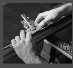
conditions, you rarely need a more acute angle than 90 degrees. If you used a 1 degree base bevel, then a 1 degree side bevel is customary. Some racers may use 2 of 3 degrees side bevel for icy conditions - usually not necessary around Montana.
