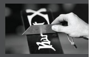
or carpenter's square could be used in a pinch. Hold the ski up to the light and look for daylight. Light showing through in the middle of the ski
