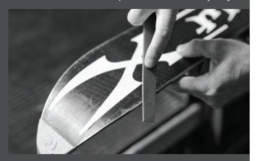
filed. Use the same soft stone to taper the edge . Begin at the front of the binding and taper to the tip. Then, work from the heel of the binding and taper to the tail. Smooth the edges slightly under foot. The goal is to have the edges the sharpest under foot and tapering in sharpness to the tip and tail. These are general rules of thumb. Try different techniques and see what works well for you.
