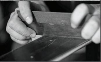
an old file to sharpen scrapers - it is best to run the scraper over the file to maintain a perfectly flat surface on your scraper. I will note here that a sharp metal scraper can be used to flatten a base-high ski. Do this only in a very limited capacity, or you can make a mess.
