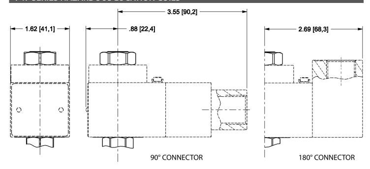
NOTE: Please verify cartridge clearance requirements when choosing a Sun manifold. Different valve controls and coils require different clearances. An additional minimum 2.0 in. (50,8 mm) beyond the valve extension is needed for coil installation and removal.
