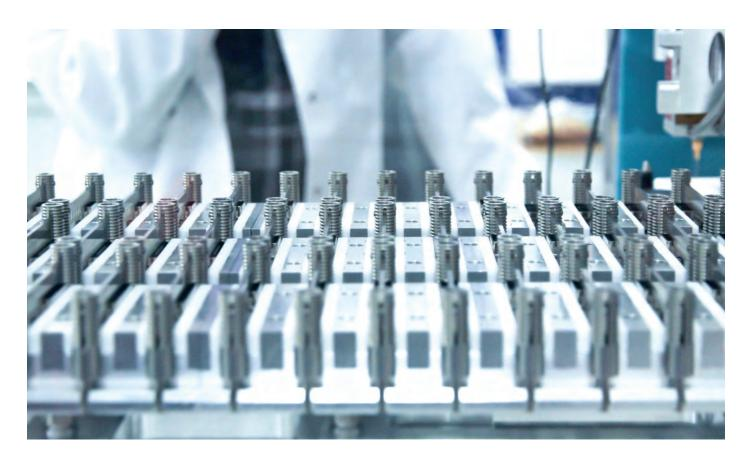
Nicomatic has automated the assembly of shell and insulator.
